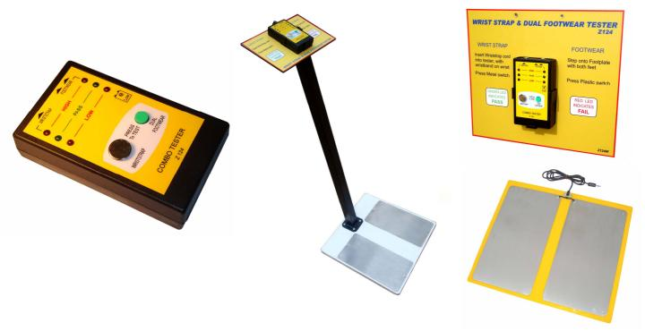
Wrist straps and ESD footwears are the first line of defence against electrostatic charge build up on the human body. They are designed to carry away this charge as soon as it is generated. At the same time the wrist strap/footwear must remain electrically safe for the user. Thus, it is important to test every wrist strap/footwear regularly.
